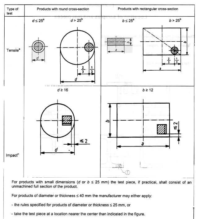
For products of round cross-section, the axis of the notch is approximately a diameter; for products with rectangular cross-section, the axis of the notch is perpendicular to the greatest rolled surface.
