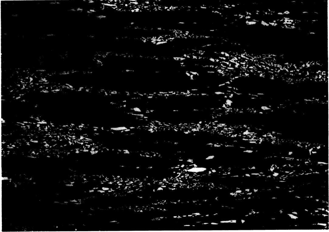
Figure 10 — Typical carbide distribution in high carbon high chromium cold work tool steel ( \times 100 magnification)
