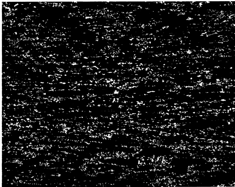
Figure 7 — Typical carbide distribution in high carbon high chromium cold work tool steel ( \times 100 magnification)
