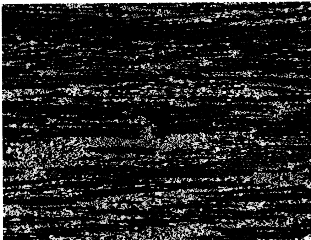
Figure 8 — Typical carbide distribution in high carbon high chromium cold work tool steel ( \times 100 magnification)
