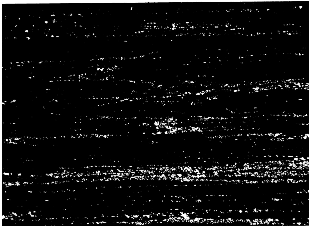
Figure 3 — Typical carbide distribution in high speed tool steel ( \times 100 magnification)
